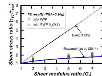
The shear stress in the stone columns is not in proportional to their relative stiffness such that the cyclic shear stress reduction due to stone columns are not significant as predicted by Baez (1995) work. The new design equation proposed by Rayamajhi et al.(2014) gives better estimate for cyclic shear stress reduction in liquefiable soil.
