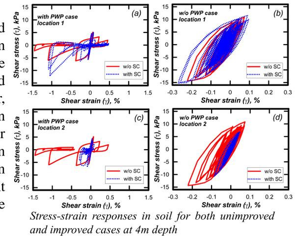
Stress-strain responses in soil for both unimproved and improved cases at 4m depth
