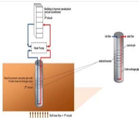
Figure 1. Diagram of energy pile by Suryatriyastuti et al (2012)
