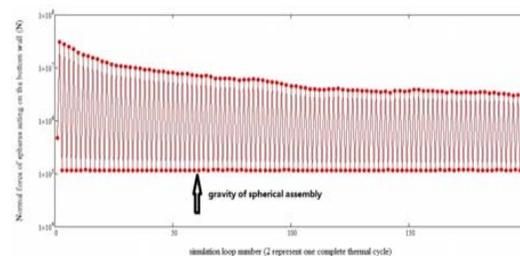
Figure 4. change of normal force from spheres acting on the bottom wall versus simulation loops (totally 200 loops or 100 thermal cycles)
