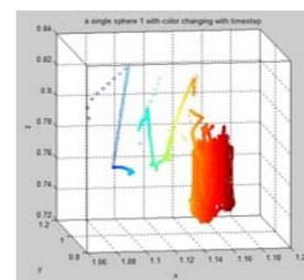
Figure 5. The displacement of one single sphere versus time (the color changing from blue to red indicates change in time)
